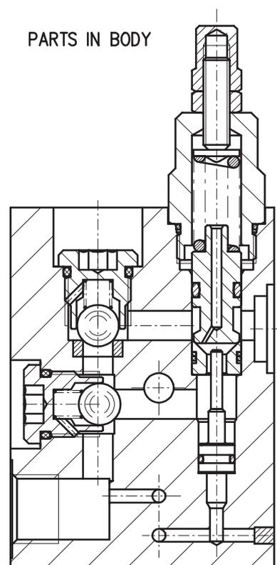
**Oil leaks from U1 (U2) to D1 (D2):** 0,25 cc/minute (5 drops) at 210 bar and 80% of the spring setting value with oil viscosity of 46 cSt.
