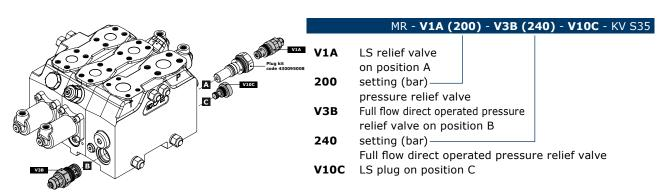
NOTE: when ordering a valve type V11C, it is necessary to specify connector type (see table "A" page 16)
